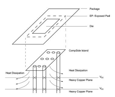
PCB Thermal Consideration for 16-Pin QFN Package (Always solder, or equivalent, the exposed pad to the PCB)
