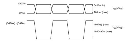
Figure 1.  $V_{\text{IS}}$  and  $V_{\text{ID}}$
