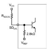
Figure 5. SD<sub>LVL</sub> Setting Circuit
